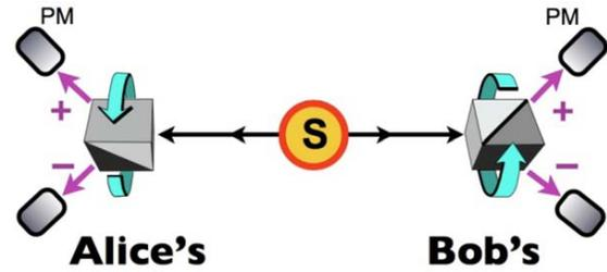
FIG. 2. (Color online) This is a conceptual diagram of a Bell test experiment with delayed choice, testing a pair of photons at polarizers. During the photons flight from the 2-photon source S, Alice and Bob rotate their polarizers to random angles  $\theta_1$  and  $\theta_2$ . Only data from the “+” side of each polarizer are used.
